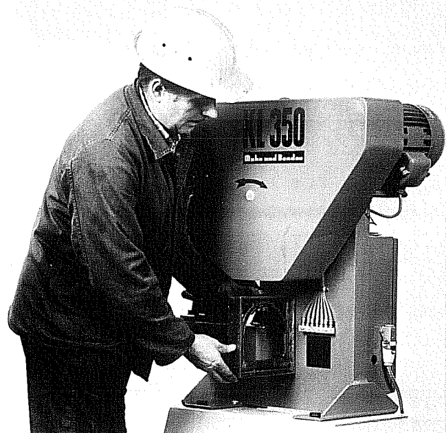
Fig. 3: Checking the position of the punch
