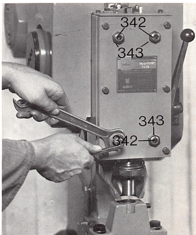
Fig.14: Adjusting the slide rails on the face side
