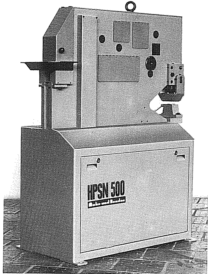
Guards on discharge side, for section, bar, and flat steel shear
