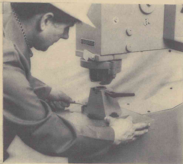
Fig. 9: Setting the punching tools
