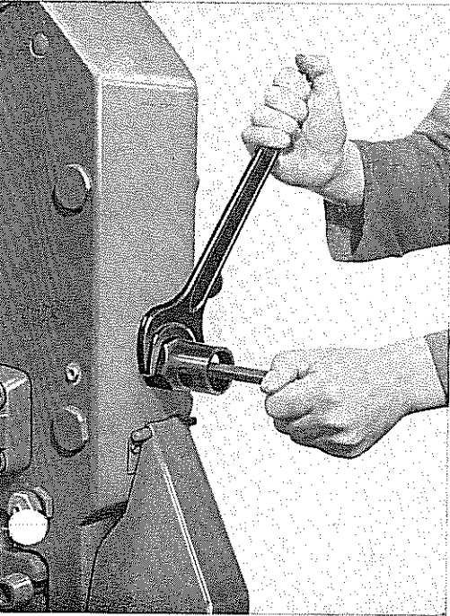
Fig. 24: Adjustment of the slide guides, upper face
