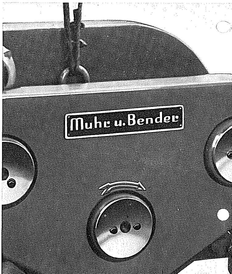
Fig. 5: Make sure flywheel rotates in the proper direction
