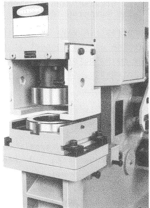
Fig. 19: Special tool holding fixture for punches and dies with cutting diameters larger than 50 mm
