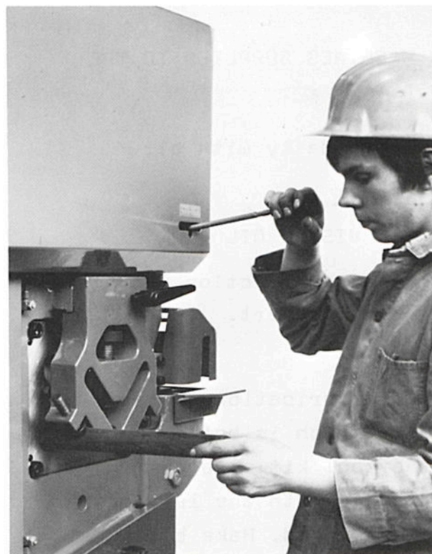
Fig. 9: Manual engagement to the shears
